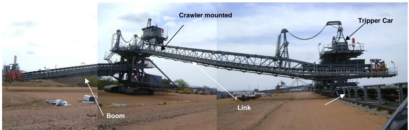
Figure 8-8: Stacker setup at Medupi Power Station
